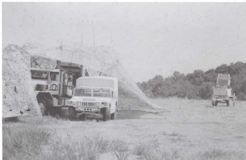
I-3 ADA Sentinel ground-based sensors can detect rotary- and fixed-wing aircraft, low-flying aircraft, unmanned aerial vehicles and ultralites in all weather conditions, 24-hours a day.
